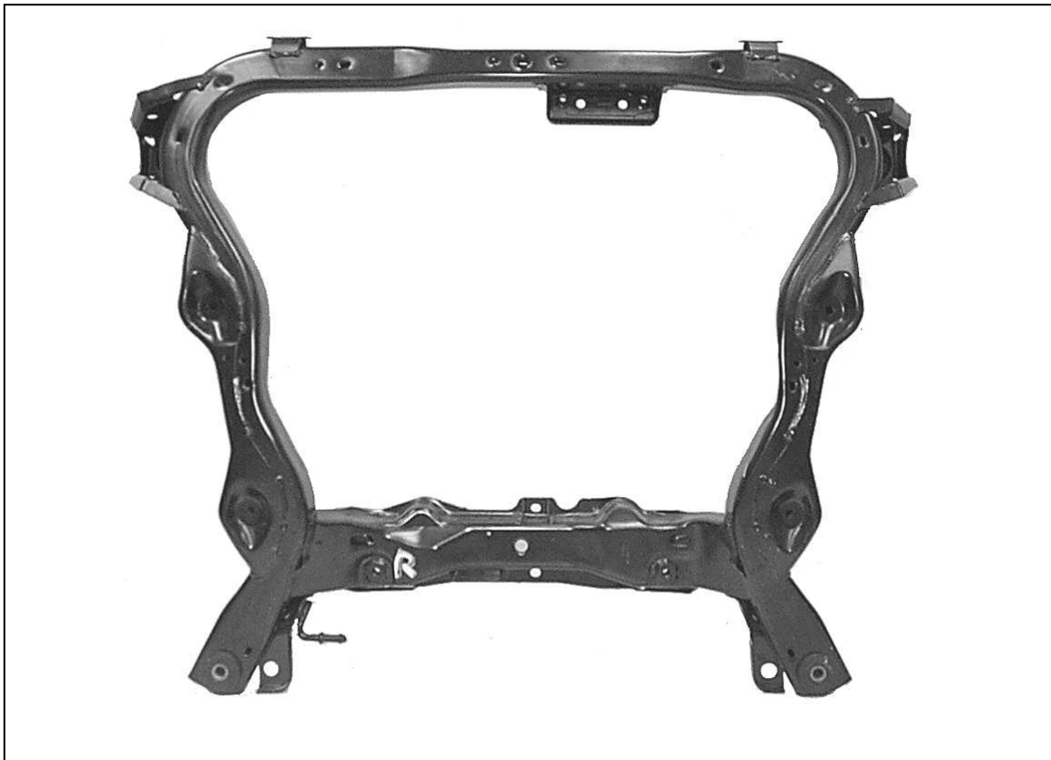
Figure 8 – Ford CDW 27 Engine Cradle Assembly
